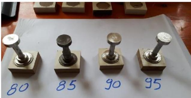
Figure 1. Samples with glued steel axes
