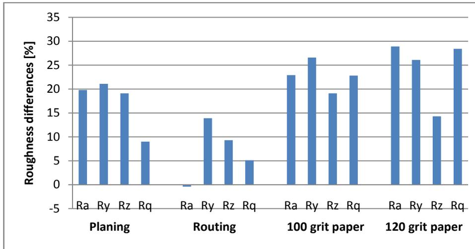
**Figure 2.** Increment of fir surface roughness referring to beech wood
