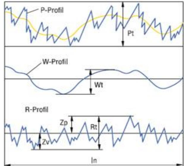
Figure 1. Separation of primary profile into waviness and roughness profiles
