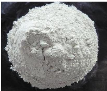
**Figure 5** Ground Granulated Blast-Furnace Slag
