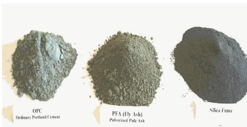
**Figure 6 . Ordinary Portland Cement Vs. Fly Ash Vs. Silica Fume**
