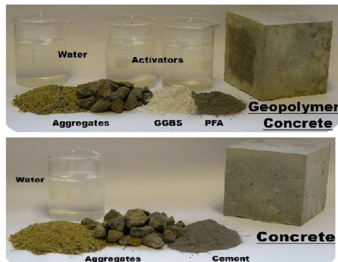
Figure 1. Ordinary concrete and Geopolymer concrete
