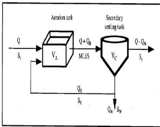
**Figure 1:** Activated sludge process
