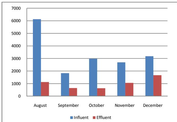
**Figure 6:** Measured of Chemical Oxygen Demand (COD) in the untreated and treated wastewater in the dairy industry
