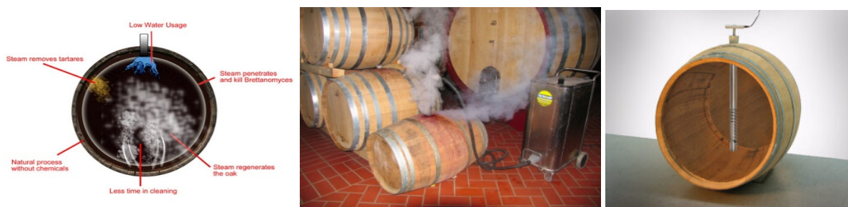
Figure 1. Cleaning, Detartrating and Disinfection of Barrels: After decanting, proceed and rinse using a high pressure machine and cold water, duration of steam cycle depending on the age and status of the barrel, proceed again and rinse with cold water.
