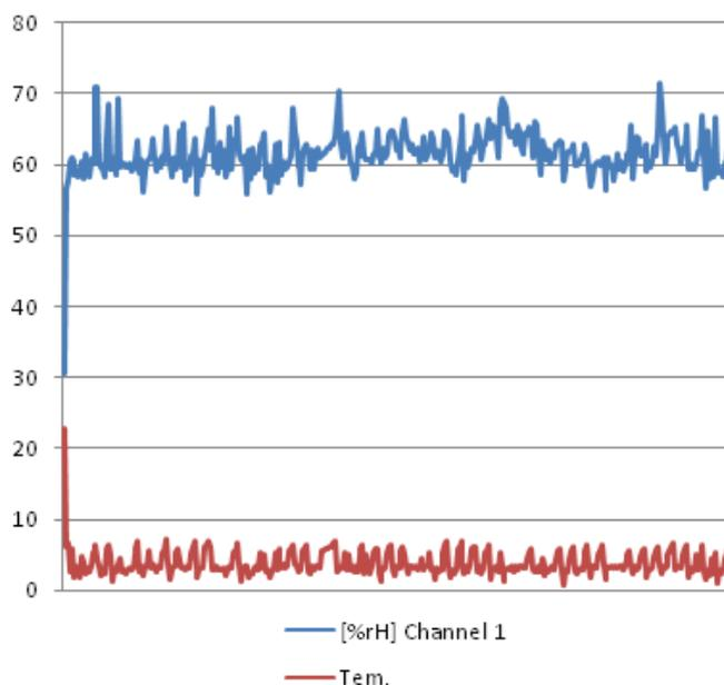
**Figure 2:** Graphical representation of temperature and relative humidity during ripening of cheese
