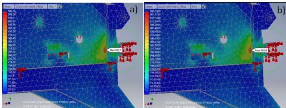
**Fig.6.** Simulation results for the variant with empty tank (a) and full tank (b). Source: own elaboration.
