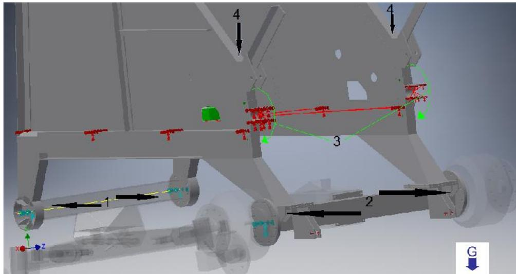
**Figure 4.** The placement of supports, forces and torques in the digital model. Source: own elaboration.
