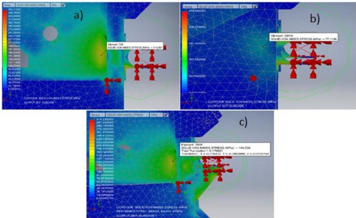
**Figure 7.** Overview graphic showing the results of static analysis conducted in the program Nastran In-CAD, for: a) angle profile, b) pentagonal profile, and c) triangular profile, which functions as a feeder house support. Source: own elaboration.
