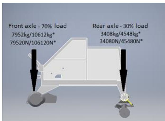
**Figure 3.** Distribution of the mass and load acting on the front and rear axle, for the variant with empty and full tank (\*). Source: own elaboration.
