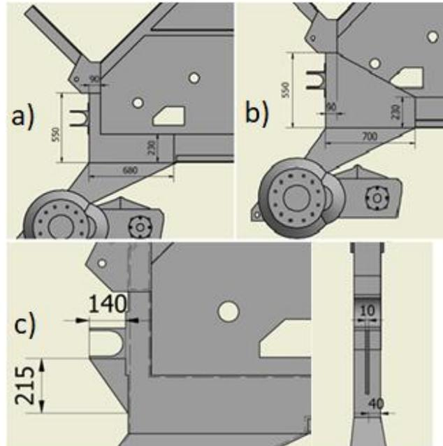
**Figure 5.** Overview drawing presenting the ideas of modification of the analyzed construction part. Source: own elaboration.
