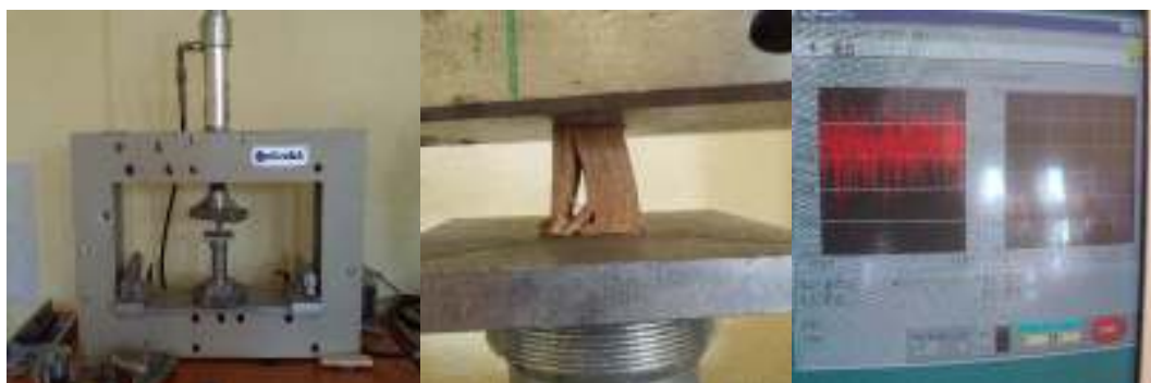
Fig 1. Tests carried out in laboratory to measure failure load during compression parallel to the grain
