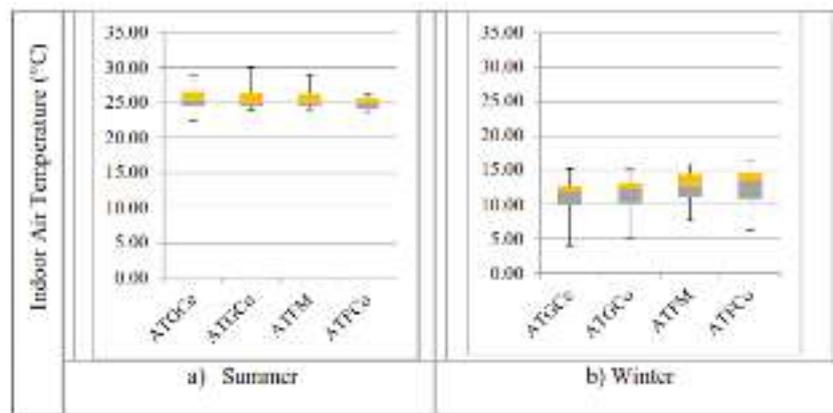
**Figure 6.** Box plot and whiskers for the indoor temperature of the window glass and wooden frame: a) summer, b) winter
