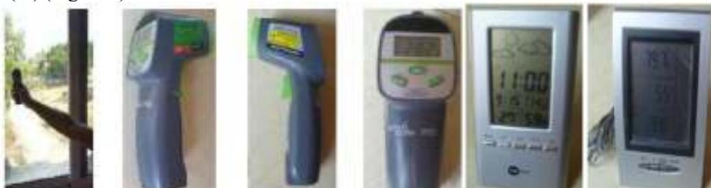
**Figure 2.** Apparatus for measuring the temperature and relative humidity of the air
