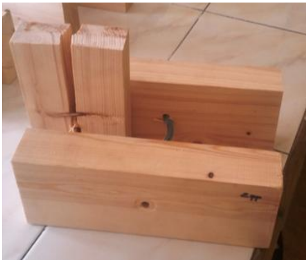
Figure 2. T-joints taken into consideration for testing
