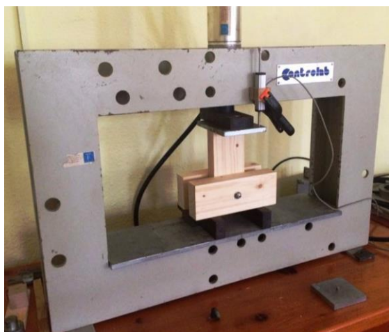
Figure 3. T-joints sample during test procedure
