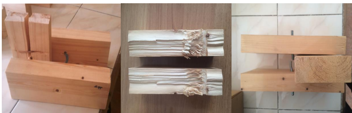
Figure 4. T-joint elemens after destruction
