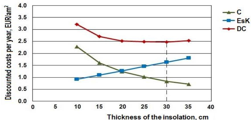
Figure 3. Dependence between the thickness of the reed roof and the relative costs in using "Donbaski" coal for fuel.
