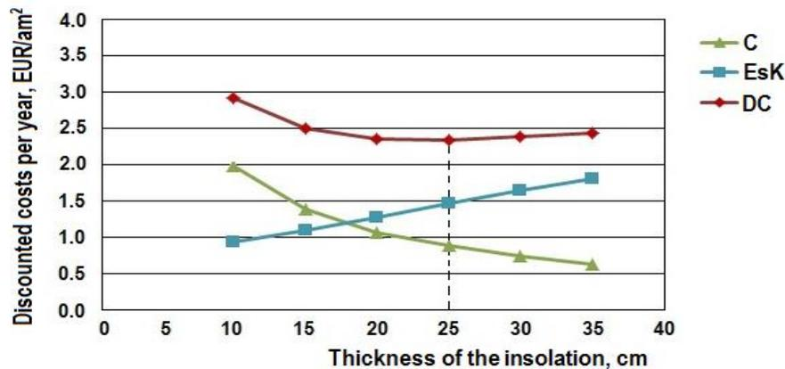
Figure 2. Dependence between the thickness of the reed roof and the relative costs in using pellets for fuel.
